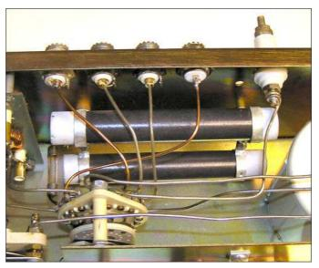
clockwise if you like. Note there is also a stop on the counter clockwise position just past the Balanced Line position. Leave it in. Please note that variations may exist. Reinstall the switch knob and hardware. You should now be able to turn the antenna switch at least one position clockwise from the COAX 1 DIRECT position. This will be the new COAX 4 DIRECT position. You can label if you like.
