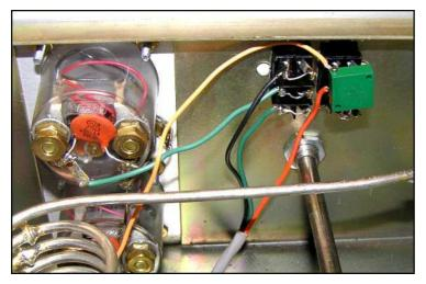
Next wire the switches. The switches I selected are DPDT. Electrically only SPDT are required. A small loop of bare wire soldered between each terminal twin provides better reliability for the low signal levels and a more secure and easy place to solder the wires and hang the trim pot.
